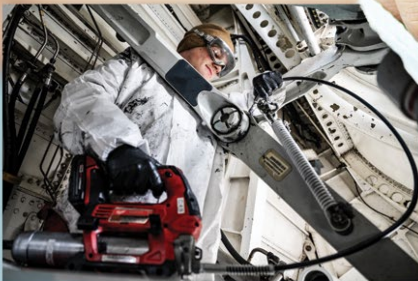
A1C Brock Thompson, 911th Aircraft Maintenance Squadron crew chief, applies lubricant to the landing gear of a C-17 Globemaster III. Photo by Joshua J. Seybert
