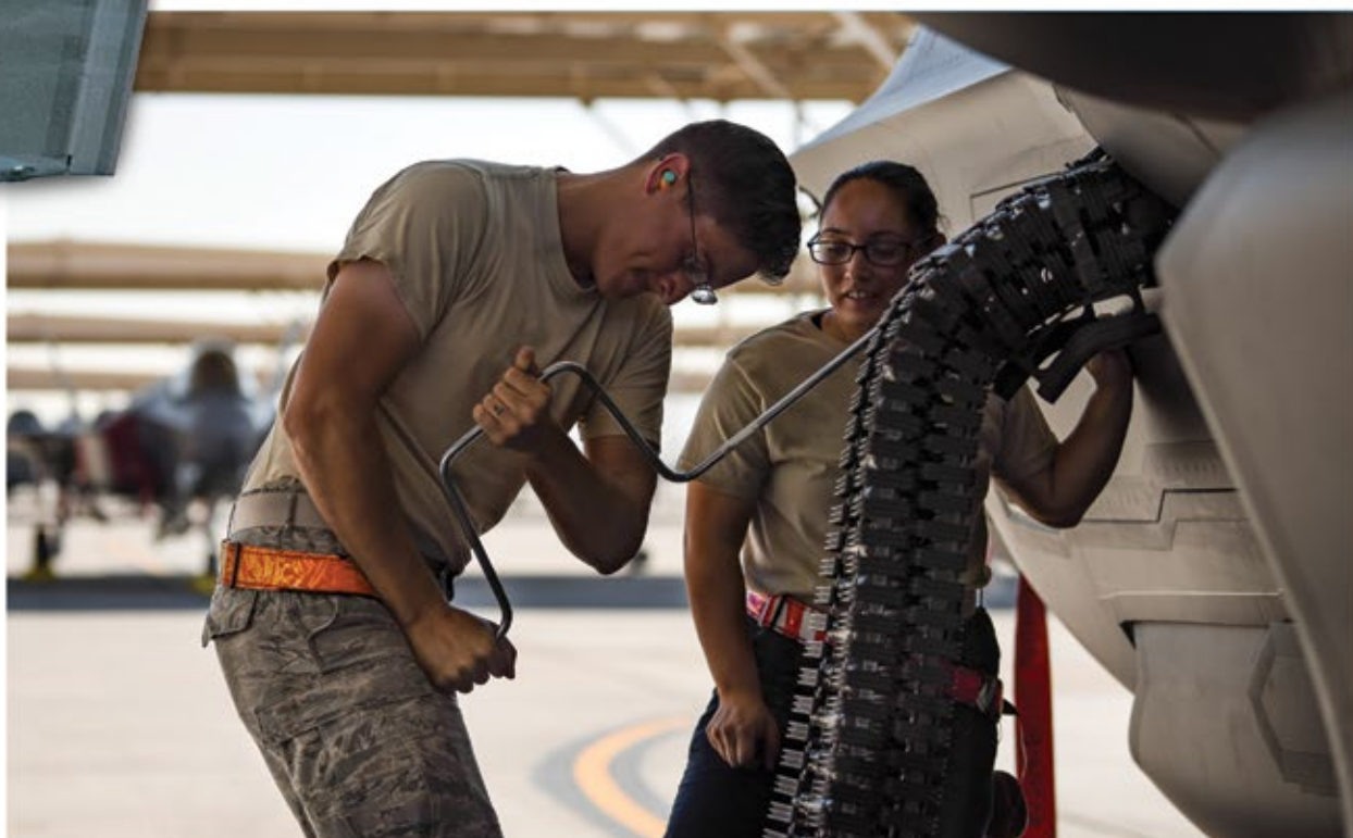
57th Aircraft Maintenance Squadron Bolt Aircraft Maintenance Unit weapons loaders attach an ammo belt (chute) to an F-35 Lightning II at Nellis Air Force Base, Nevada. Photo by A1C Andrew D. Sarver
